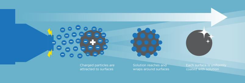
Electrostatic sprayer technology works by sending a positive electric charge through the sanitizing solution, causing it to be attracted to negatively charged surfaces like two poles of a magnet. This technology removes the liability of human error from the sanitizing process.
